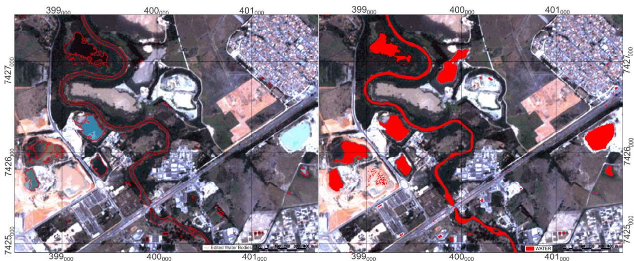
Fig. 7 - A portion of the Jacareí image, with the R3G2B1 enhanced color composition overlaid by the edges of the Paraíba do Sul River and sand mining lakes from the K-Means classification (left), and the classification result from the NDWI thresholding (right).
