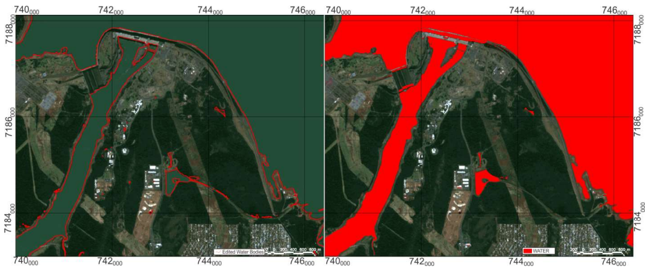
Fig. 8 - A portion of the Foz do Iguaçu image, with the R3G2B1 enhanced color composition overlaid by the edges of the Paraná River and the Itaipu reservoir from the K-Means classification (left), and the classification result from the NDWI thresholding (right).
