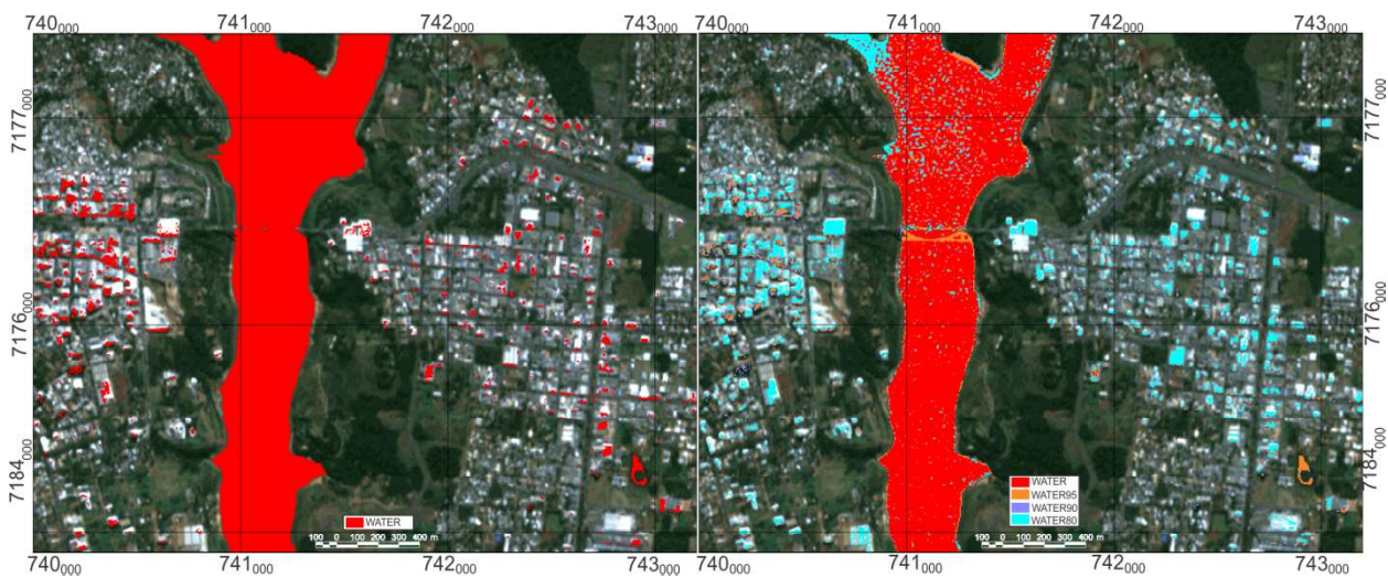
Fig. 12 - Comparison between classification using MNDWI (left) and using Hue component from the R2G3B5 color composition (right) for a region in Foz do Iguaçu image.
