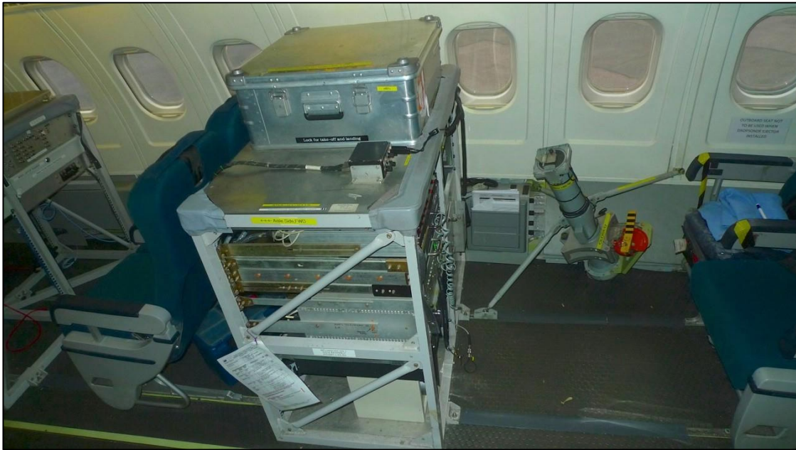
Figure 3.4 AVAPS/LIDAR rack and the dropsonde launch tube.
