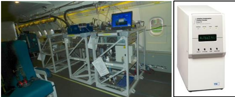
Figure 3.9 The CPC/CCN Rack (left) and the condensation particle counter (right).
