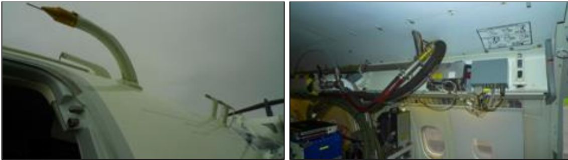
Figure 3.12 Low turbulence inlet (left) and Interior components in the cabin (right)
