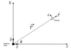
Figure 1. Reference system for Central force problem
