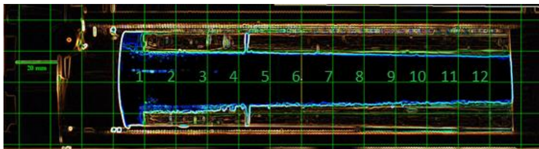
Figure 5. Illustration of a processed image used to determine the diameter variation along the grain's length.
