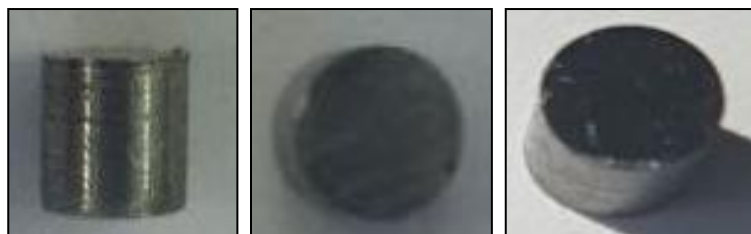
Figure 2. Samples prepared of SAE 1020 Steel
