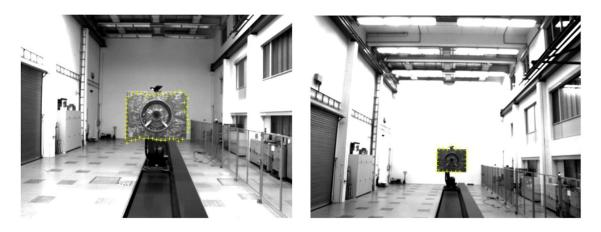
Figure 6.13 - Tracking edges of the target mock-up at 10 m (left) and 20 m (right).
