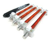
Figure 2.10 - An illustrative example of magnetic torqrods. Source: Space Research on Unique Technology (2014).
