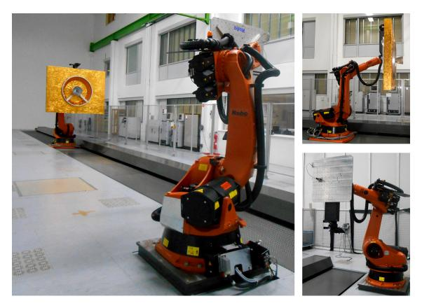
Figure 6.1 - The robots of the European Proximity Operations Simulator (EPOS).
