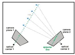
Figure 2 – Two cameras with epipolar constraints
