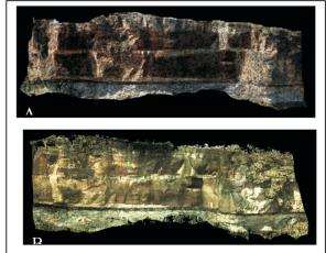
Figure 7 - 3D Reconstruction from photos (A) and terrestrial laser scanner (B).
