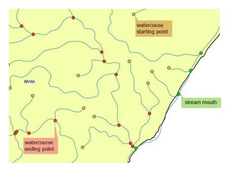
Figure 1. Kinds of Points in Drainage Network
