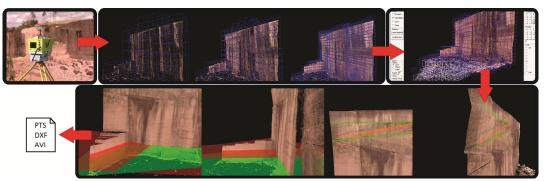
Figure 3. Field data acquisition using a terrestrial laser scanner, processing, editing, interpretation, and exportation of a digital model based on point cloud.
