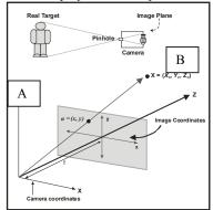
Figure 1 – Pinhole camera (A), Model (B)
