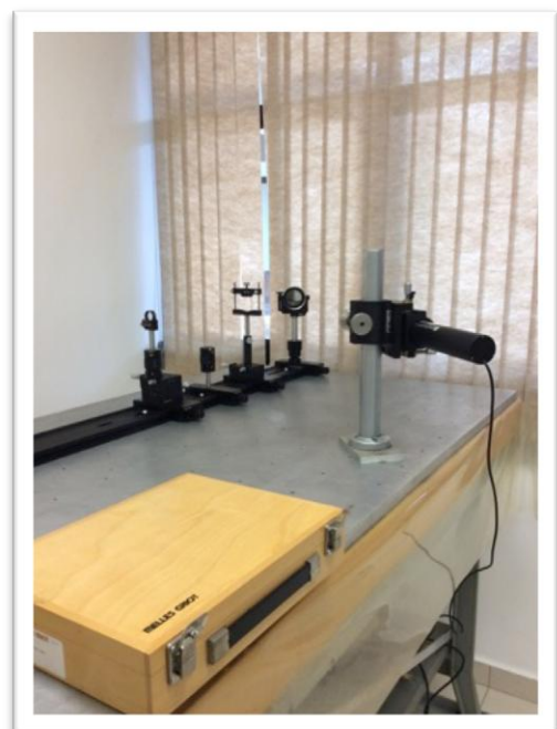
Figure 22: The images show a very simple setup for the solar projection on a cabinet at the room 10 in the second floor of the INPE's Building CEA II.
