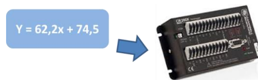
Figure 4. Offset adjustment and multiplier factor applied to a datalogger used in a weather station
