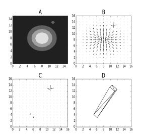
Figure 2 – Example of GPA operation sequence, starting from matrix image (A): the gradient field (B),the asymmetric gradient field (C), and the triangulation(D). In C we can see  $N_v = 6$ , and in D we can see  $N_c = 10$ , then according to the equation 2,  $G_A = \frac{10-6}{6} \approx 0.6667$
