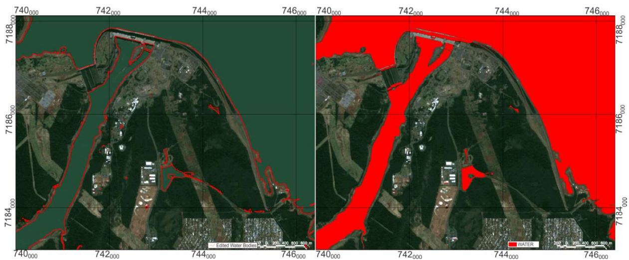
Fig. 8 - A portion of the Foz do Iguazu image, with the R3G2B1 enhanced color composition overlaid by the edges of the Paraná River and the Itaipu reservoir from the K-Means classification (left), and the classification result from the NDWI thresholding (right).
