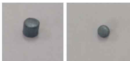
Figure 5. Sample T4-2 with mill scale a) frontal view b) top view
