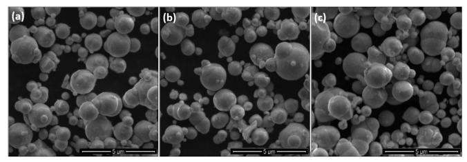
Fig.2 FEG-SEM images obtained for the three particulate sizes with 15.000 of magnifications of (a) 25 < Pe < 53, (b) 53 < Pe < 63, and (c)  $Pe > 63 \mu m$ .
