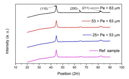
Fig.3 X-ray diffractograms of CI samples as a function of particle size (a)  $25 < Pe < 53 \mu m$  (b)  $53 < Pe < 63 \mu m$  (c)  $Pe > 63 \mu m$  (d) without sieving
